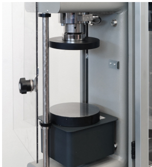
Fragment guard for flexure station (50-C99/P) fitted with door switch (50-C50/P1)
